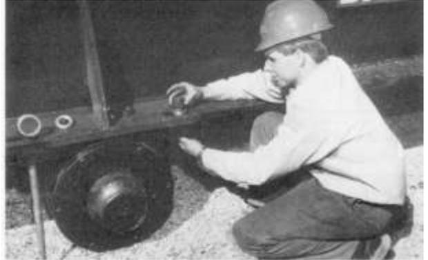
**Step 3:** To align the center bearing measure the distance from the front of the walking beam to the center of the center bearing shaft. When measurements on both sides are equal, tighten the bolts securely.
