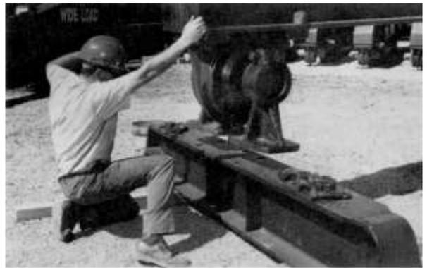
**Step 2:** Select the pitman arm which has the lubrication line attached to it. Note the position of the lubrication line on the equalizer. The two should be assembled so that the lubrication lines are on the same side.
