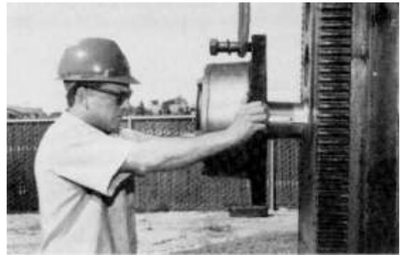
**Step 4:** Using the box end hammer wrench, tighten the crank pin nut as tight as possible by hand. This will establish the metal to metal position for the final tightening procedure.
